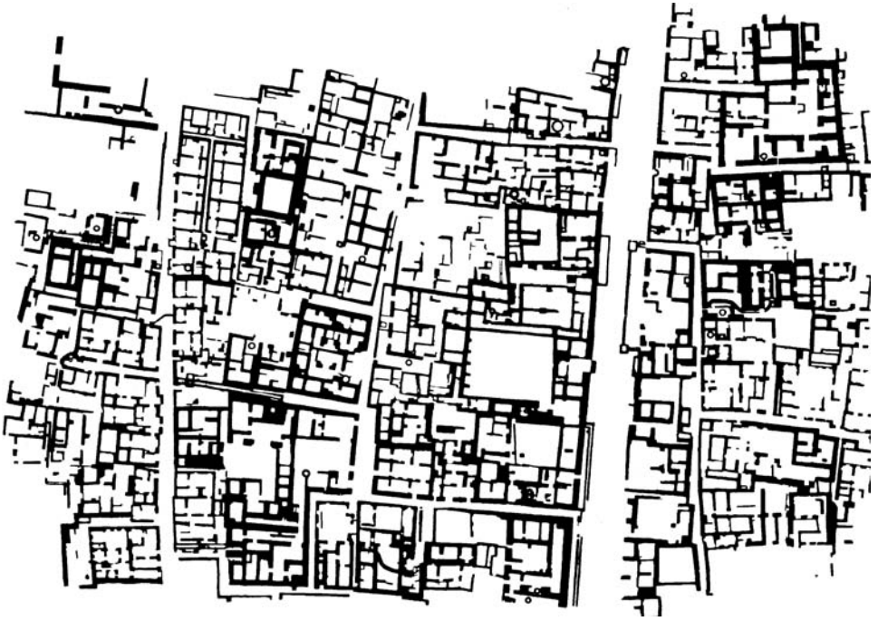
Figure 8: Residential Zone of Mohenjo-Daro, a Harappan City in Pakistan, Showing Semiorthogonal Urban Blocks
